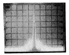
Fig. 3 — Synthesizer noise about the carrier. Vertical divisions are each 10 dB; horizontal divisions are each 20 kHz. The transceiver was being operated at rated input power on the 20-meter band.
