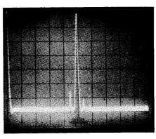
Fig. 1 — Spectral display of the FT-757GX. Vertical divisions are each 10 dB; horizontal divisions are each 5 MHz. Output power is approximately 100 W at a frequency of 24.7 MHz. All spurious emissions are at least 55 dB below peak fundamental output. The FT-757GX complies with current FCC specifications for spectral purity.
